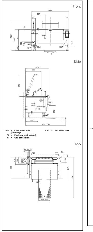
Front 1600 581 160 160 8<u>1</u> đ ļ 1254 700 900 250 42 HAIK 195 EI CVI G Ш ΤT Side 1014 680 **7**' 965 걥 50 Т 550 min 1750 CWII HWI = Hot water inlet Cold Water inlet 1 (cleaning) = EI = Electrical inlet (power) G = Gas connection Тор HWI G 260 315 355 900 971 750 y -R min 500
